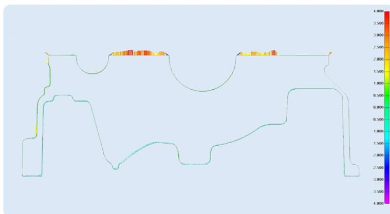
—→ Radial measurement (2D cross section)
