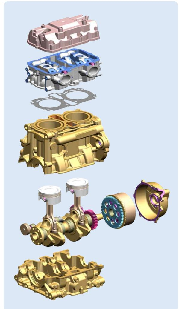
—→ Exploded view of combustion engine components including the crankcase to be inspected
