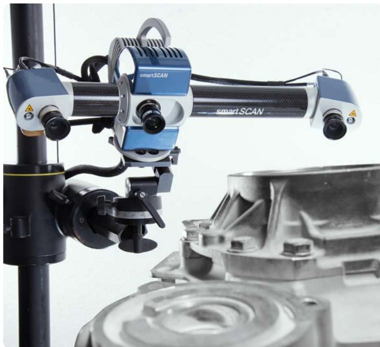
—→ 3D scanning of a gear transmission casing
